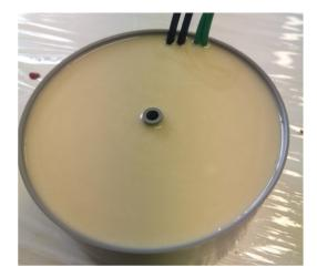
**VUKOL N34** is a medium hard, but still flexible material, containing inorganic fillers. It is characterized by considerable mechanical tensile strength, flammability class V0/4mm, thermal conductivity 0.6 W/(m.K). Very well adhesive to metal surfaces. It can be hardened with the hardener VUKIT LV or VUKIT M. With VUKIT M, the material with VUKIT M is slightly harder as a result.
