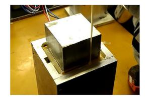
**VUKOL N70** is a medium-hard, flexible material with a high content of mineral fillers. The substance is highly adhesive to metals, mechanically strong, has good thermal conductivity (0.75 W/(m.K)), flammability class V0/4mm (UL certified).
